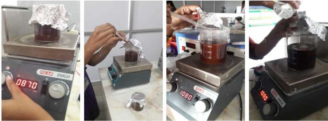
Figure 2: Series of steps involved in synthesis of magnetic nanoparticle by co-precipitation method
