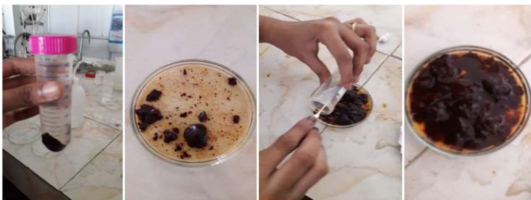
Figure 4: The magnetic nanoparticles are centrifuged and dried using microwave oven
