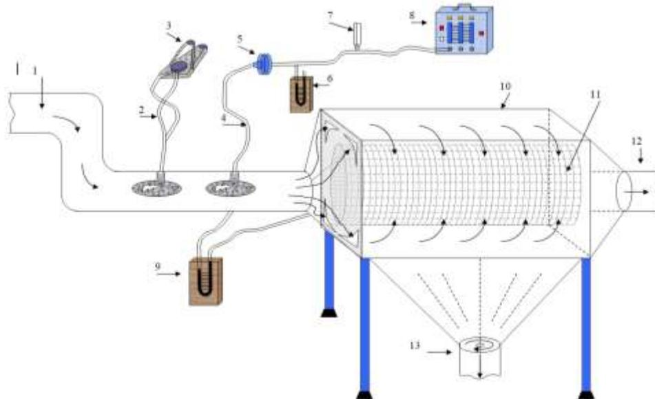
Figure 1: Energy-Saving Simple Dust Collector: 1 - Inlet Pipe; 2 - Pneumatic Tube; 3 Micromanometer; 4-Pipe for Collecting Dust; 5-Filter AFA; 6-Manometer; 7-Thermometer; 8-Aspirator; 9-U-Shaped Pressure Gauge; 10-Case; 11 - Small-sized Metal Mesh; 12-Outlet Pipes; 13-bin for Garbage
