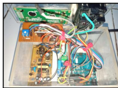
Figure 13. Wiring Arduino to WiFi module ESP 8266-01
