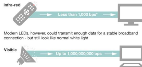
Fig. 2. How LiFi sends data [8]
