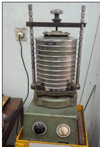
Fig. 1: Sand Distribution Machine
