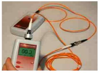
Fig. 10. Light Source and Power Meter. Source: FOA
