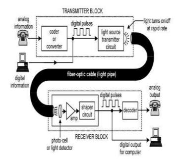
Fig. 4. Fiber Optic Communication Block Diagram
