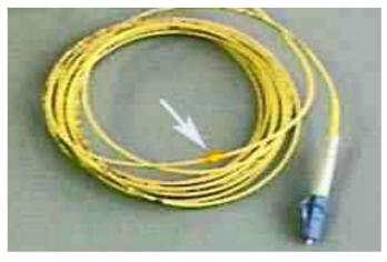
Fig. 9. Visual Fault Locator Source: (FOA)
