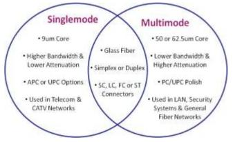
Fig. 3. Fiber Modes Comparison. Source: Cables-solution.com
