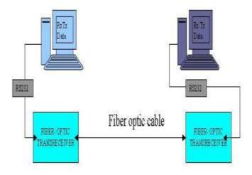
Fig. 5. Fibre optics for PC to PC Communication. Source: FOA (Fiber Optic Association Inc.)
