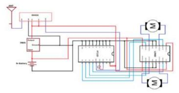
(a) Circuit diagram of the receiver section
