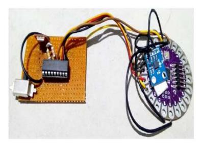
(b) Implementation of Arduino Lilypad with transmitter section
