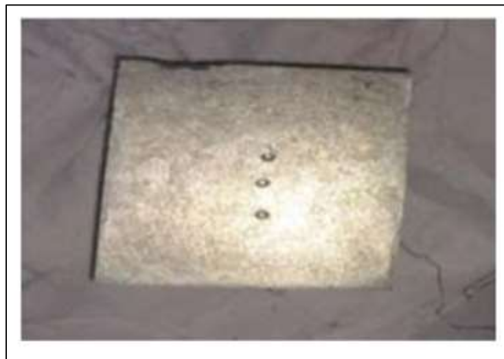
Figure 4. Fig.3-specimen 2(TiB2 10%, AA7075 90%)
