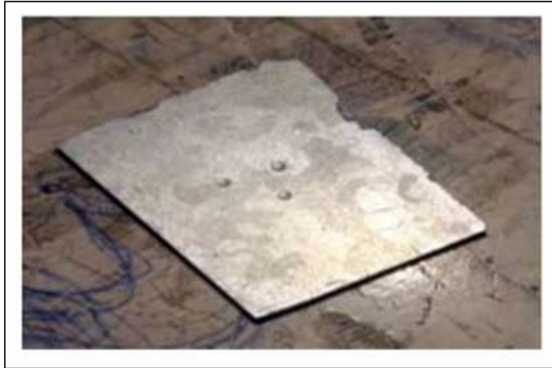
Figure 3. Specimen 1(TiB2 5%, AA7075 95%)
