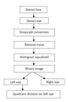
Fig. 6: Processing Structure of the Proposed Method
