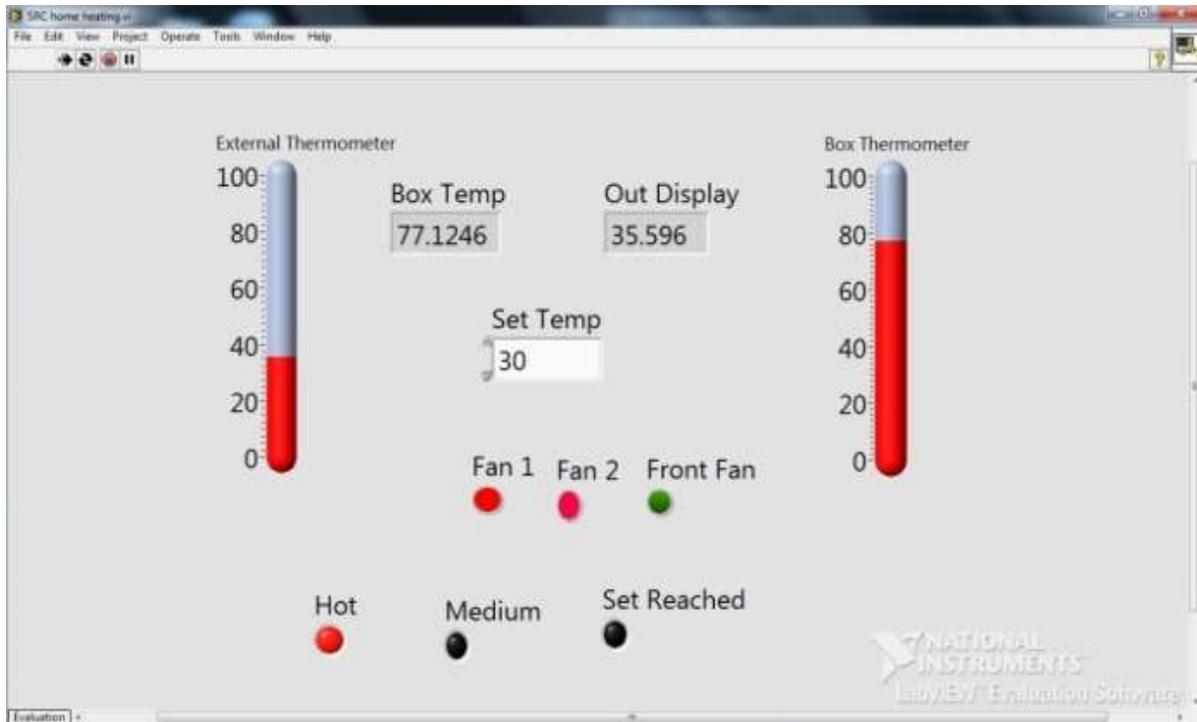
Fig. 12: Front Panel of MHC setup in VI for hot condition
