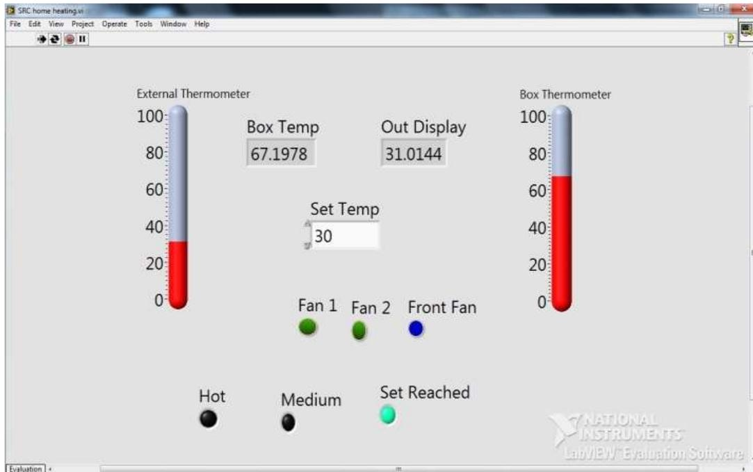
Fig. 10: Front Panel of MHC Setup in VI for Set Point Condition
