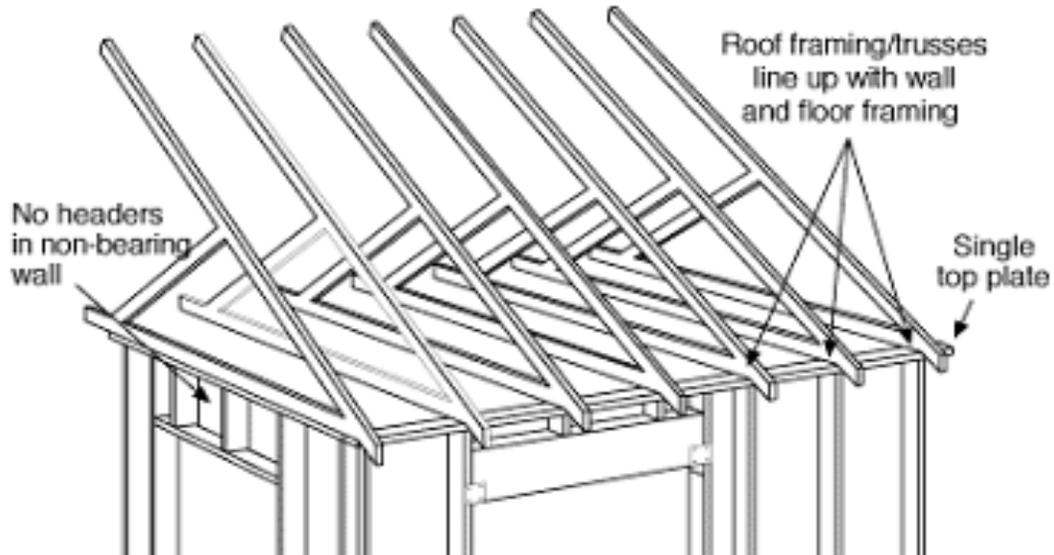
Figure 2: Advancement Framing on In-Line
