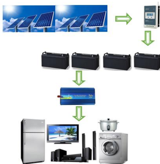
Figure 1: the solar power generation systems for households used in research
