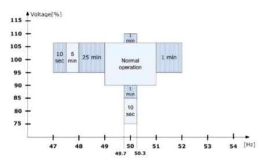
Figure 18. Voltages versus frequencies plot for a wind turbine
