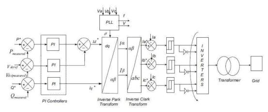
Figure 6. Control of Synchronous voltage oriented using PI controllers.
