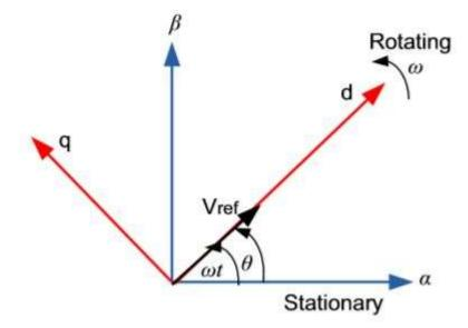
Figure 17. Synchronous rotating reference frames.
