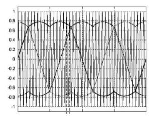
Figure 14. Triangular carrier SVPWM.
