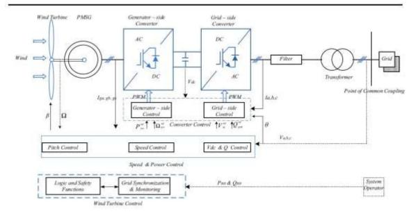
Figure 1. WECS overall controlling levels.
