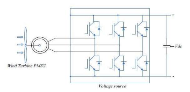
Figure 2. WECS organization of machine side converters.
