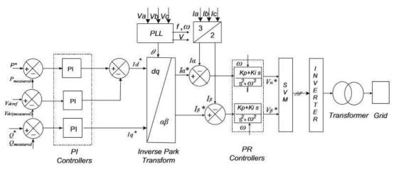
Figure 7. Stationary VOC with proportional resonant controller.
