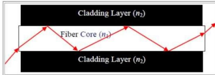
**Fig. 1: Simplified diagram showing light propagation through optical fiber (cladding region has lesser RI as compared to core region, i.e.  $n_2 < n_1$ ).**
