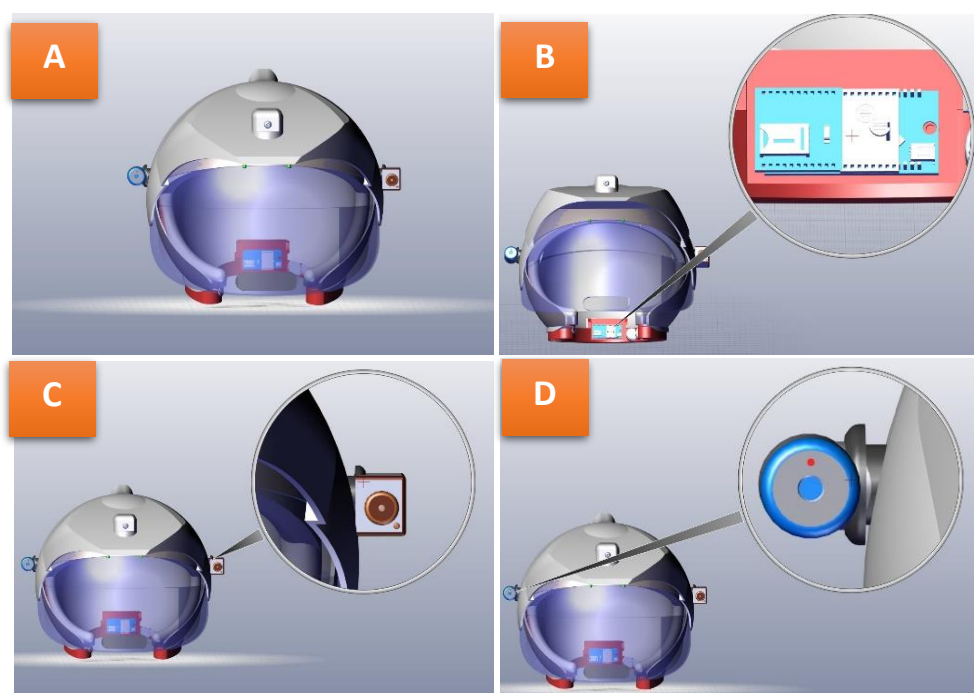
Figure 4: configuration design of the system (a) Over all system, (b) System Controller, (c) Thermal Camera and (d) Optic Camera.
