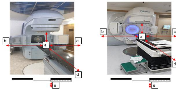
**Figure 4. Measuring position of OSLD (a) Beam center(SSD 100 cm), (b) Left 250 cm, (c) Right 250 cm
