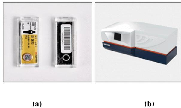
**Figure 2. Dosimeter and reader (a) OSLD (b) Auto200**
