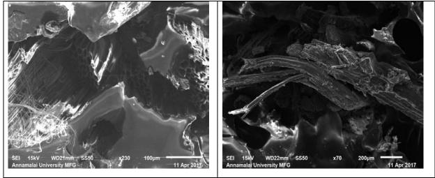
**Figure 9:**(a & b) The SEM Micro-graphs of the surface of untreated Sisal fiber reinforced epoxy composite
