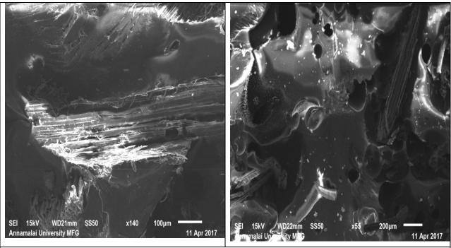
Figure 10:(a & b) The Micro-graph surface of Sodium hydroxide Treated Sisal fiber reinforced epoxy composite
