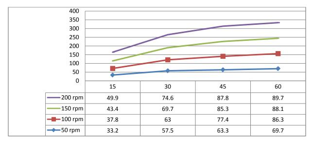
Fig. 3. Results of studying the influence of basket rotation speedon the intensity of the release of diclofenac sodium from Dikomz capsules
