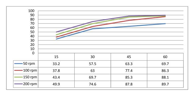
Fig. 4. Results of studying the influence of basket rotation speedthe intensity of the release of omeprazole from capsules "Dikomz"
