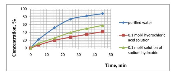
Fig. 2. The results of a study of the effect of pH of a solvent on dissolution rate of capsules "Dikomz" (omeprazole)
