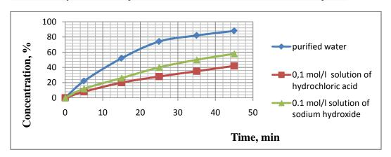
Fig. 1. The results of a study of the effect of pH of a solvent on dissolution rate of capsules "Dikomz" (diclofenac sodium)
