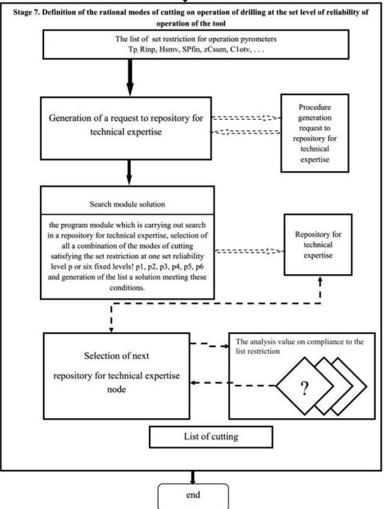
Figure 2. Sequence of Definition of the Modes of Cutting providing the set probability p trouble-free operation of the axial tool in the presence of the limiting factors.
