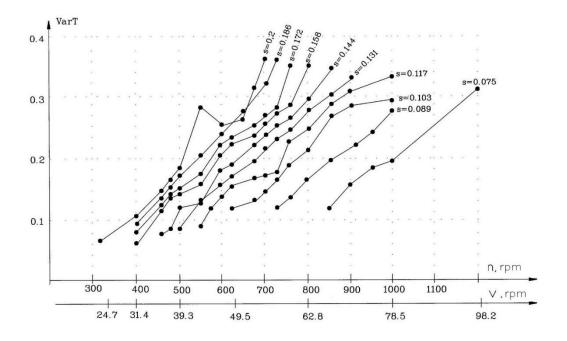
Figure 1. Dependence of a variation of firmness of drills on the cutting modes. Results of simulation modeling of processing of structural steel( $\sigma_{R}$ =610 MPa; HBo=2235 MPa; VarHB=20%) pointed drills with plates from BK8
