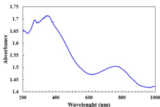
**Figure 10:** UV-Vis absorbance of  $Ti_3C_2$
