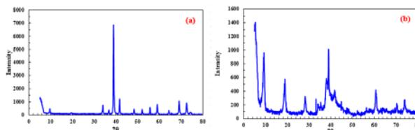
**Figure 5:** XRD pattern of (a):  $Ti_3AlC_2$  and (b): incomplete etching of  $Ti_3AlC_2$  in lower concentrations (10%, 20% and 30%)
