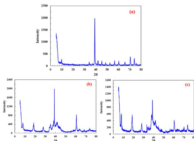
**Figure 8:**XRD pattern of powder resulted from in-situ HF solutions in (a) 25 °C, (b): 40 °C and (c): 50 °C
