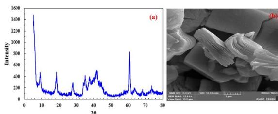
**Figure 7:** XRD pattern and FESEM image of etched  $Ti_3AlC_2$  with HF 40% and 60 h
