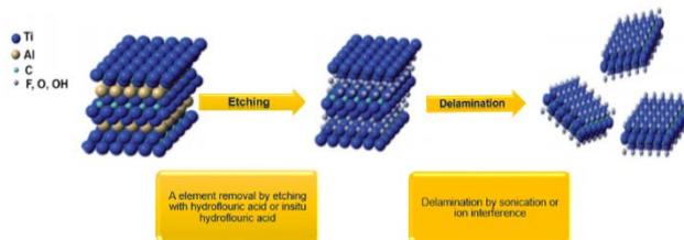
**Figure 4:** Schematically illustration belonging the chemical etching of  $Ti_3AlC_2$
