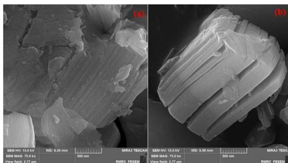
**Figure 6:** SEM images of (a):  $Ti_3AlC_2$  (b):  $Ti_3C_2$  achieved with lower concentrations
