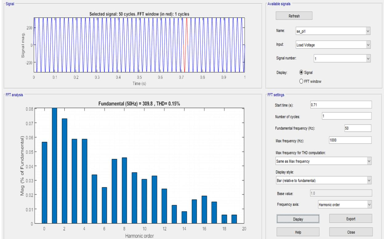
Figure 9: THD Analysis of the proposed system Voltage
