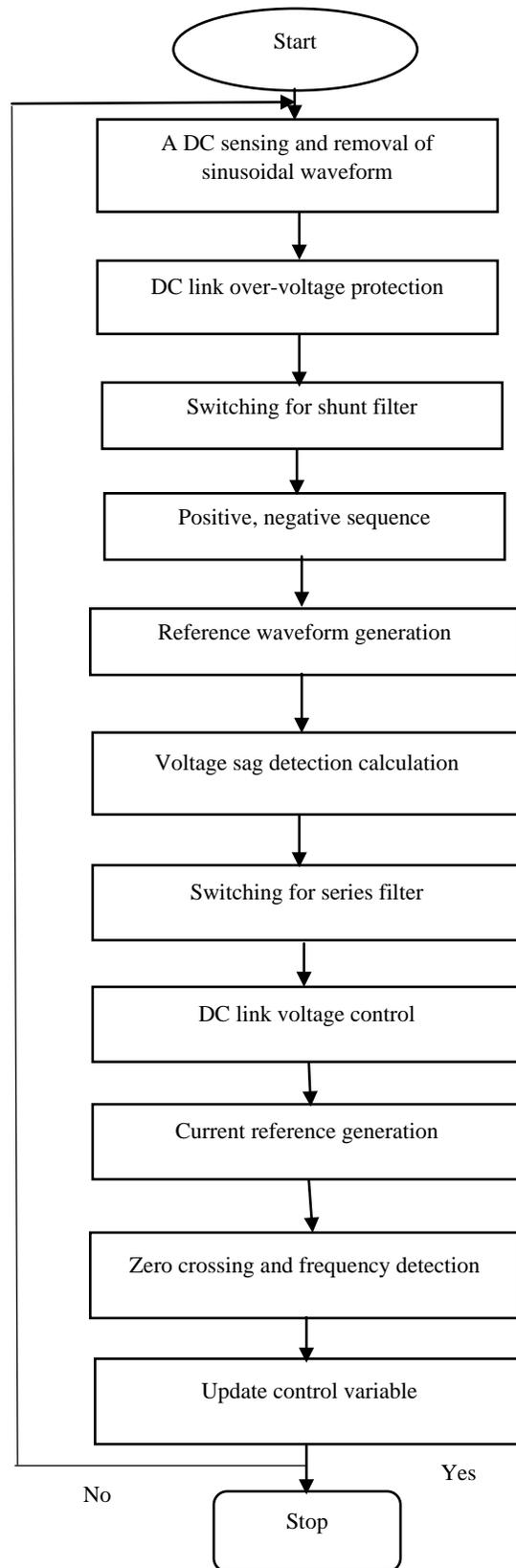
Figure 5: Proposed Power Impelling Optimization Technique(PIOT)Flowchart
