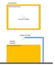
Figure 10:Design of Sensor Placement in Garbage Container.
