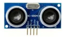
Figure 4:HC-SR04 Ultrasonic sensor type[7].
