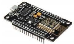
Figure 1:NodeMCU ESP8266[5].
