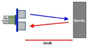
**Figure 3**: *How to Work Ultrasonic*[7].
